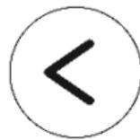
**short press** – scroll between home screens to the left, select widget menu if menu bar is pulled up, scroll up in menu, lower value during setting parameter, **press & hold** to rapid value lowering
