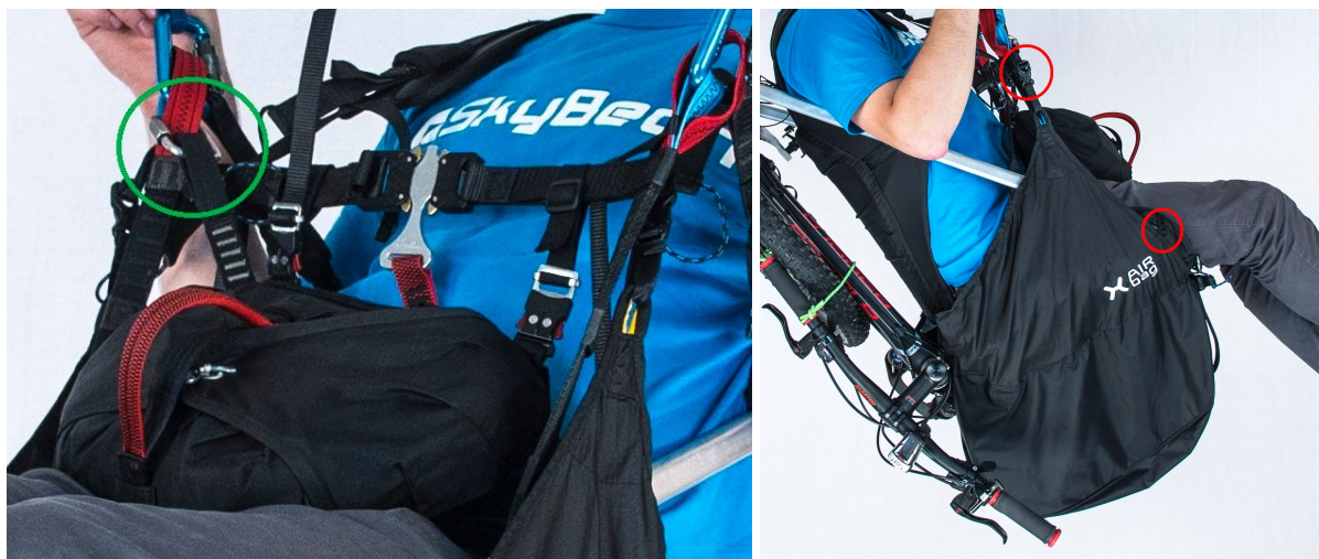
Picture 6: Reverse parachute attachment and airbag connection
