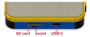
Except SD card slot opening, there are two more ports on the bottom of vario
